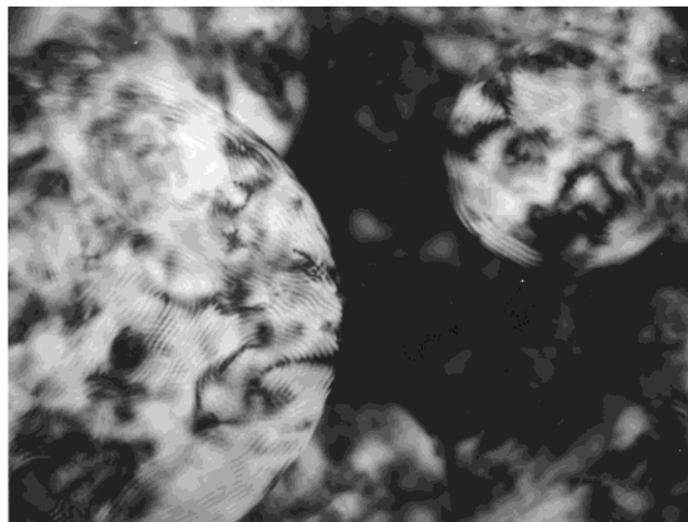
Figure 3. PSLG/dodecane solution containing liquid crystalline spherulites with cholesteric banding bathed in dark, isotropic phase. Image spans \sim 2 mm in the horizontal dimension.
